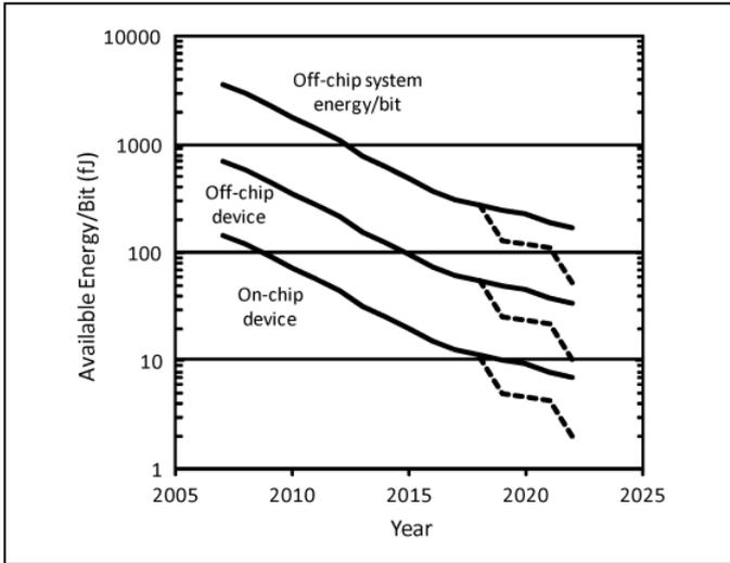
Figure 1. Projected evolution of the chip communication requirements in terms of energy per bit (extracted from [1])
