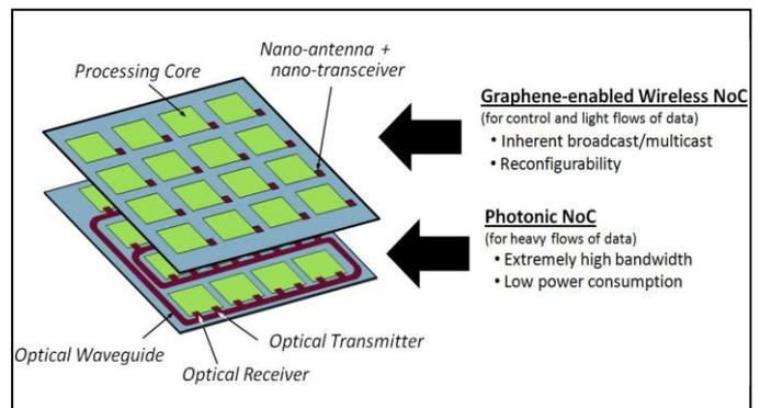
Figure 2. Example of a graphene-enabled hybrid wireless-optical NoC
